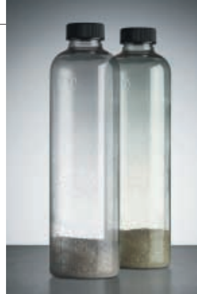
AA scavenger additive (used in bottle on left) improves color and addresses AA-related taste and odor issues.
