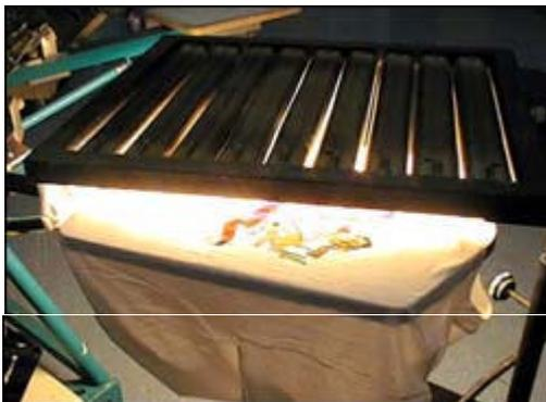
*A word of caution. If you use an electric dryer, the thermostat control will turn your heat panels off and on. Record the dryer readings during both stages of on and off, make sure your dryer stays above the recommended temperature even when it is on the low side. The goal of the flash unit is to help the ink reach the gel phase.*
