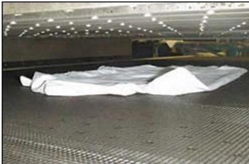
*The ink film temperature is actually rising slowly as it passes through the oven, and it usually doesn't hit the high temperature until it is close to the end of the oven.*
